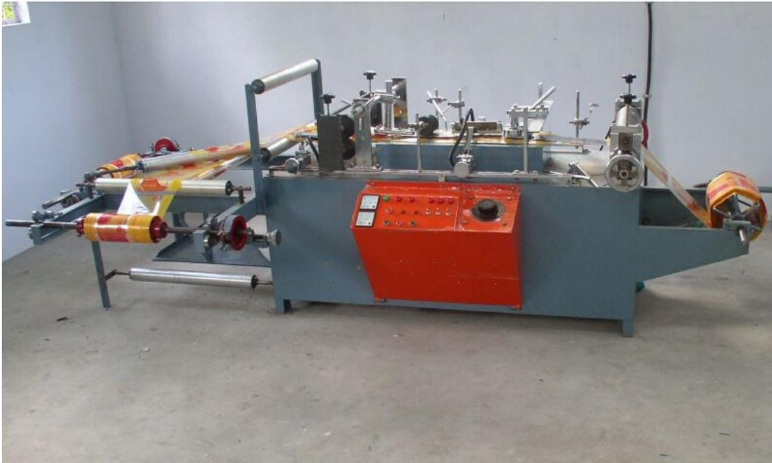
**Suitable to make pouches from heat seal able poly laminate substrates like Polyester-ploy, BOPP, Glosinpoly etc.**
