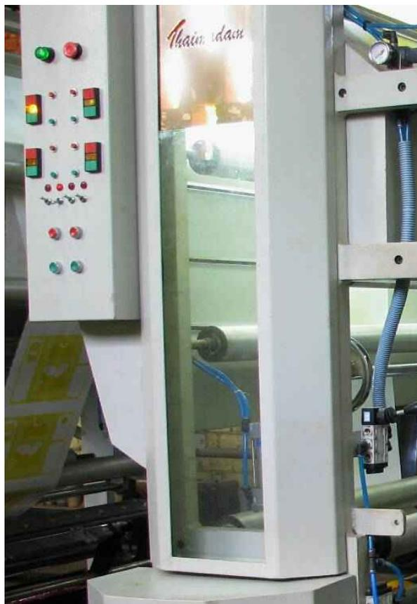
In the conventional machines, the operator has to sit down and look upwards, leaning inside the machine to get a view of the printed format or the doctor blade assembly if anything goes wrong the operator has to face a lot of troubles to get a clear picture of this situation. Almost all the upper area constituting drying chamber is enclosed and cannot be seen from outside. This problem is completely eliminated in Thaimadam Machines.
